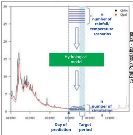
Figure 2. Theory behind the prediction of low flows using hydrological modelling (Premhyce).
